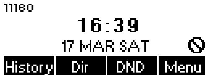
Figure 56 - DND Enabled on All Lines
